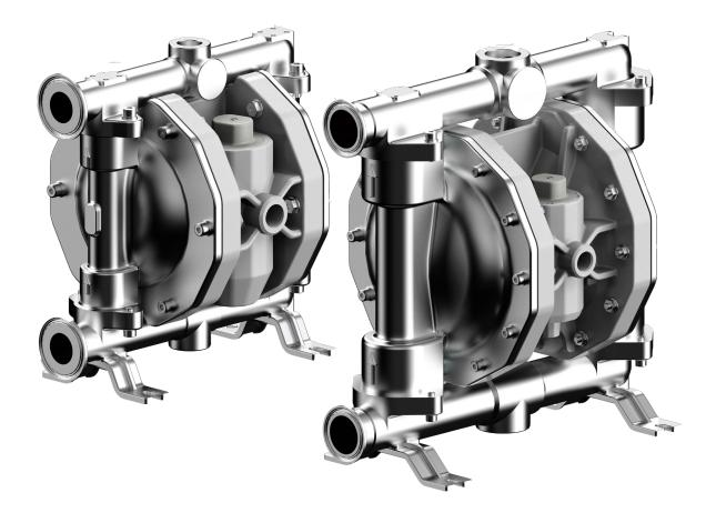
**ASTRA "SP"** diaphragm pneumatic pumps are manufactured fulfilling FDA requirements. All materials in contact with the liquid are realized according to FDA requirements. The whole range is in AISI 316 electro-polished according to the International Provision ASTMA380 and the medium roughness is 2,7  $\mu$ m.
